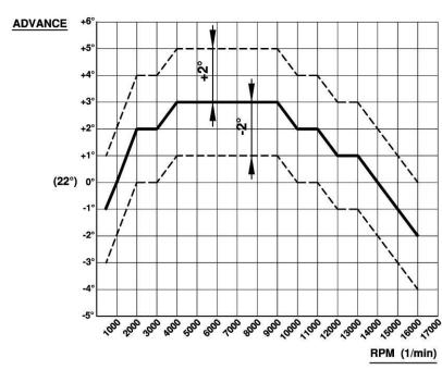
THE ZERO INDICATION ON THE DIAGRAM MEANS WHEN THE REFERENCE ON ROTOR AND STATOR MATCH EACH OTHER.
