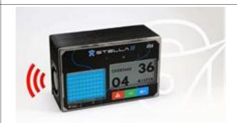
When the competitor ahead considers passing is appropriate and safe. He must press the blue button. This action will turn off the alert sound and his LEDS monitor in blue colour will change from being flashing to steady.
