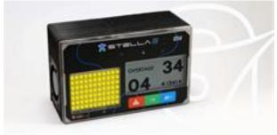
Your request has sent an alert to the vehicle ahead and his LEDS monitor will start flashing blue, followed by an alert sound or beep. This condition will continue until the competitor ahead authorizes the pass.
