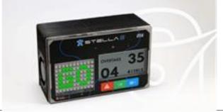
At the moment you will be able to pass in a safe way. This generates immediate reports and, in case of block that impedes passing, the race management will be informed. It is not recommended to overtake or pass if the word "GO" doesn't appear on your monitor.
