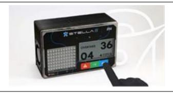
Your LEDS monitor will flash in yellow colour to indicate that the vehicle you are attempting to pass has not received your request for passing. When the yellow monitor stops flashing, it indicates that the vehicle ahead has already received your request for passing.
