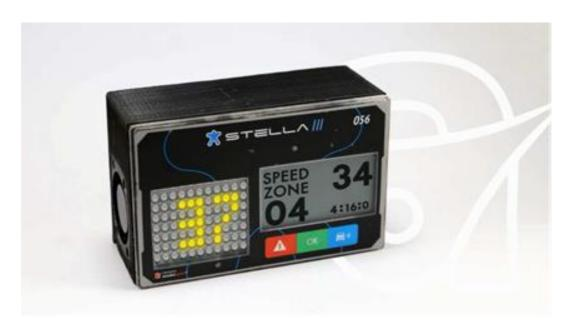
Upon entering the speed zone, the speed limit will change from flashing yellow to steady red color on your LEDS monitor.
