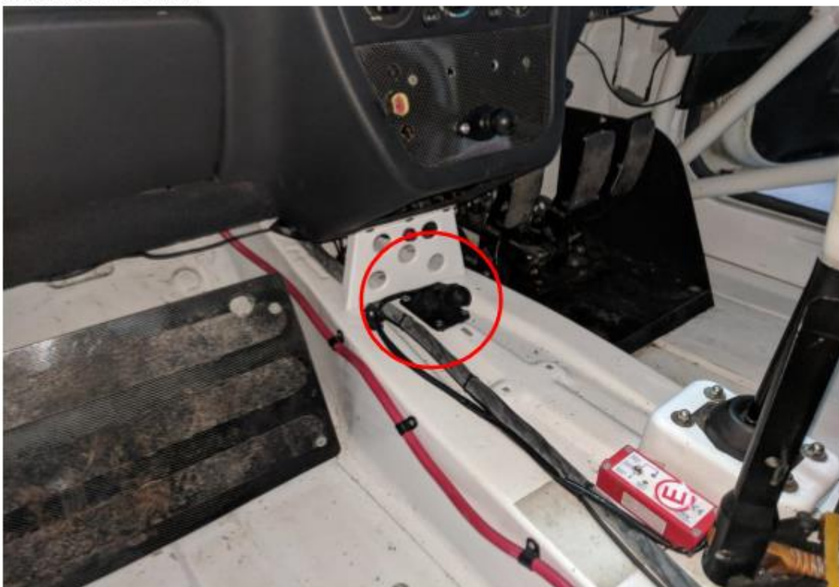
Here the 25mm rubber ball mount is securely attached to the tunnel.
