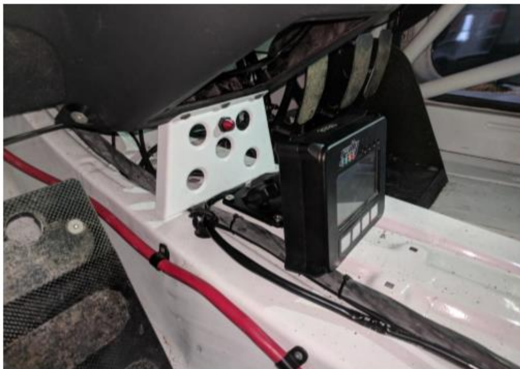
The WRC tracking unit then mounts to the 25mm rubber ball mount (connected through the RallySafe connector).
