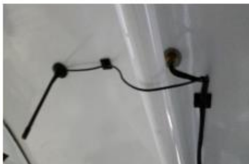
Here the antenna is stuck to the inside centre of the roof (Preferred)
