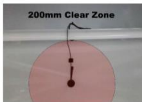
Please note the internal antenna must be 200mm AWAY from any roll cage components
